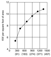
Figure 72A. Minimum air velocity required for ULTRA-SAFE<sup>TM</sup>, feet per minute (meters per minute)
