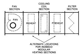
Multi-Zone or Dual Duct Heaters – These heaters are designed for installation inside multi-zone or dual duct air conditioning equipment, where the airflow is highly variable and unevenly distributed (Figure 52). These heaters use coils derated to approximately 25 watts per square inch (3.8 watts per square cm) of wire surface area (approximately one half normal watt density). Low density coils run cooler and thus provide longer life under these stringent operating conditions.
