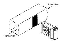
Figure 86B. Optional Slip-in Heater Installation
