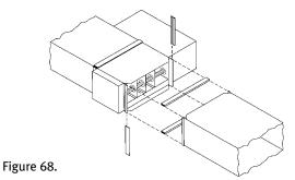
This option for custom flanged heaters, allowing installation with conventional HVAC slip-and-drive connections, offers the rugged and secure mounting of a flanged heater, yet requires less installation labor than a slip-in heater. It is particularly useful when other equipment in the duct system uses slip-and-drive connections, as the contractor can standardize throughout (Figure 68).
