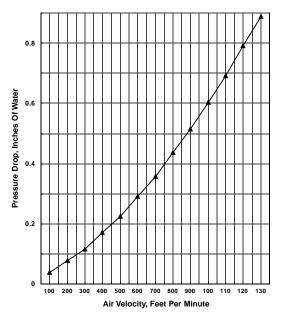
Figure 72D. ULTRA-SAFE™ Pressure Drop Curve
