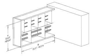
Figure 71. Flanged Duct Heater
