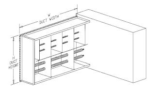
Figure 70. Slip-in Duct Heater
