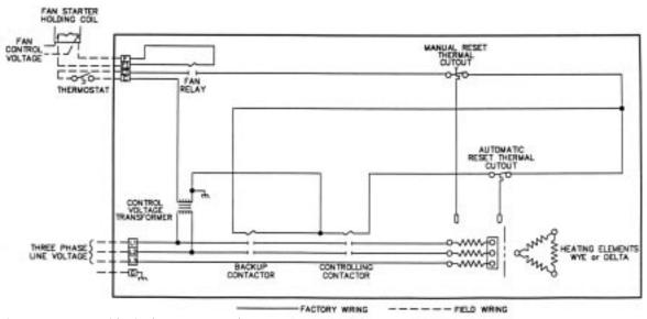
Figure 77. Heater with Single Stage Control
