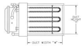
Figure 83. Dimensional Drawing for EP2
