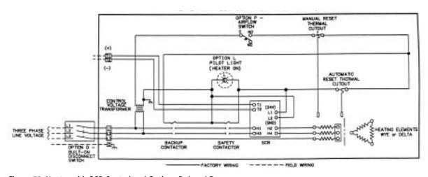
Figure 78. Heater with SCR Control and Options D, L and P
