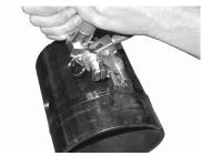
3. Roll tool over as far as tool will go, and push forward cutter handle. Remove tool and tap down ears of clip to complete clamp. Remove excess material from winding mandrel.
