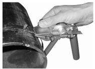
1. With the Bantam Tool in the Pistol Grip Position, Place the band in the tool with sufficient band in the winding mandrel.
