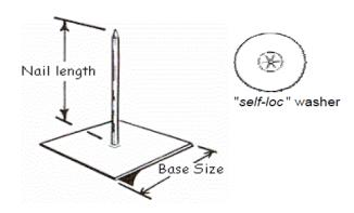
Self Adhesive hanger pins are used to secure insulation /liner inside air-conditioning or heating ducts.
