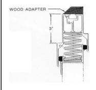
If the condenser section is supported by a separate pedestal beyond the standard roof curb, a separate aluminum spring rail or multiple OSM-1 isolators are provided to support this overhung section.
