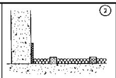
ROLLOUT ISOLATION MATERIAL LAY PLYWOOD POURING FORM SLOT FACING TOWARDS MOUNTS FOR HIGH LOAD AREAS AND CONNECT EDGES USING las detailed in drawings.
