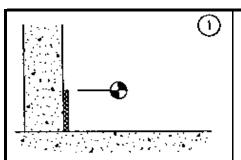
STRIKE FLOATING SLAB GRADE. NOTE: PERIMETER BOARD SET AND ADHERE PERIMETER BOARDS TO ALL CURBS AND PENETRATIONS.
