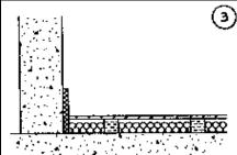
WITH MOUNTS AND ACOUSTIC SHEETS ON TOP OF ISOLATION BLANKET, INSERT ADDITIONAL MOUNTS, STAGGERING JOINTS JUNCTION PLATES AND SCREWS
