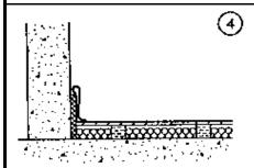
INSTALL TWO LAYERS OF POLY FILM OVER FLOOR, EXTEND UP AND OVER PERIMETER ISOLATION. SEAMS SHALL BE OVERLAPPED 4" AND CONTINUOUSLY TAPED TO PREVENT AGAINST CONCRETE LEAKAGE.
